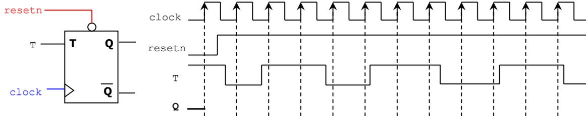
b) Complete the timing diagram of the circuit whose VHDL description is shown below: (5 pts)
